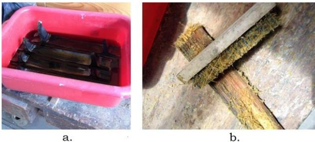
**Figure 4** (a) Samples submerged in sodium hydroxide. (b) Sample brushing process.
