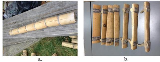
**Figure 2** (a) Guadua residues obtained for the test. (b) Guadua divided in internodes.
