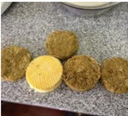
**Figure 5** Finished fiberglass and guadua fiber samples.
