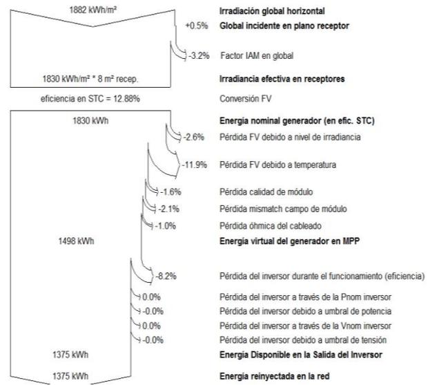
**Figure 8** Sankey Diagram of annual losses based on PVsyst simulation
