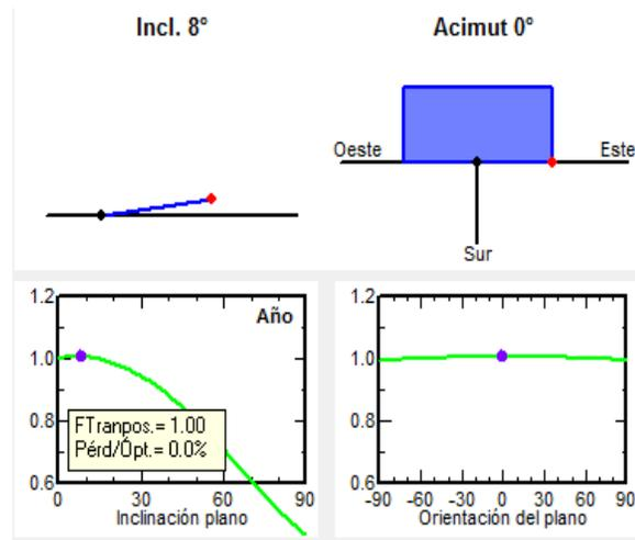
Figure 2 Orientation of photovoltaic modules
