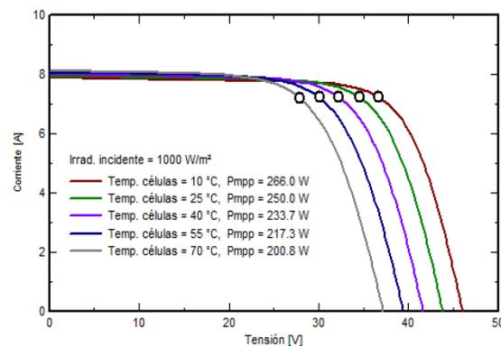
Figure 4 Performance of the module based on incident irradiance and temperature (Source: PVsyst)
