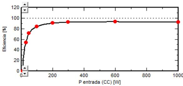
**Figure 5** Efficiency of the 1kW grid-tied inverter. Source: PVsyst
