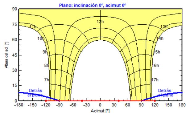
Figure 3 Sun path and horizon profile
