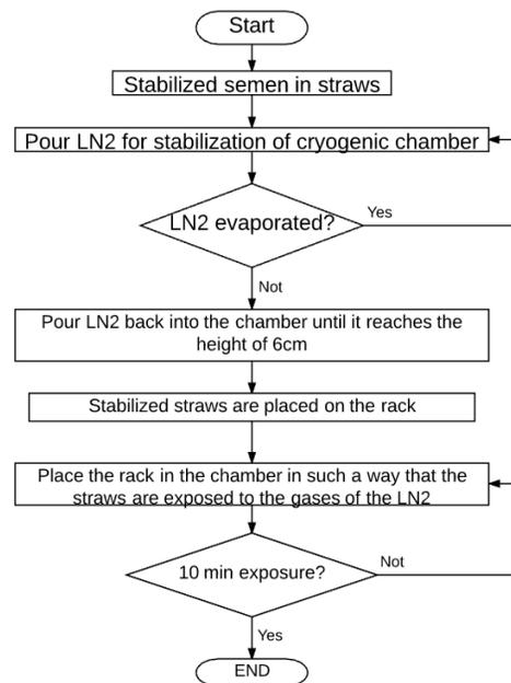
Figure 4 Current procedure used to freeze bovine semen.
