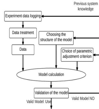
Figure 10 Flowchart of experimental identification process.
