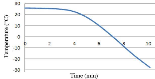
**Figure 16** Freeze rate at 66 psi.
