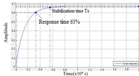
Figure 13 Response to the P-type controller step function.
