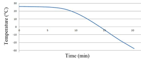
**Figure 15** Rate of freezing at 33 psi.
