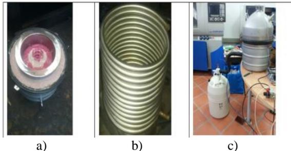
**Figure 7** a) Cryogenic chamber of custom tank, b) Coil for uniform distribution of temperature, c) Tanks coupled together ready for tests.
